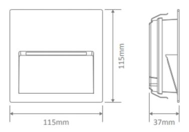
Cutout without recessed box: (L) 100mm x (W) 100mm Cutout with recessed box: (L) 110mm x (W) 110mm
